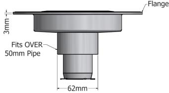
Connection to pipe must be primed and solvent welded.
