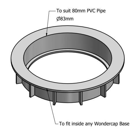
80mm Grate Adaptor fits any size Wondercap Base and will accept 80mm Grate or can be flipped to accept 80mm PVC Pipe.
