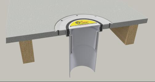
Reduce your waterproofing problems by simply rebating the outer flange into the subfloor prior to waterproofing.
